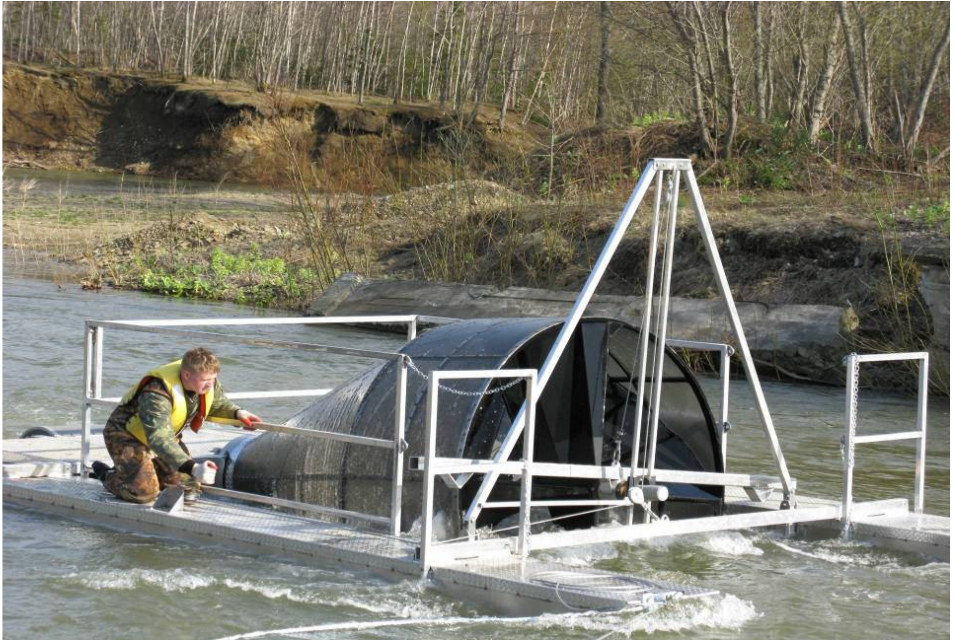
Test of rotary-screw trap
