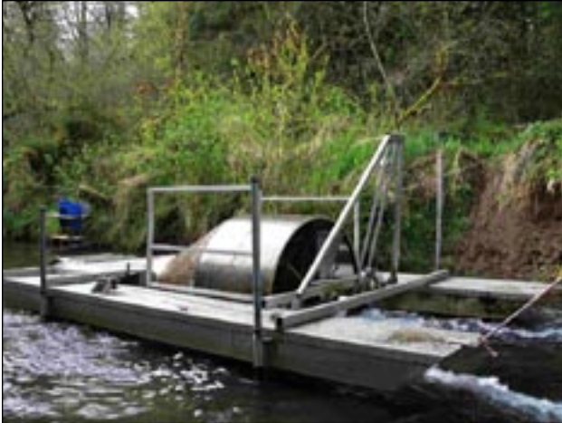
FIGURE 15. — Rotary screw trap in operation during low stream flows with the pontoon barge supported above the water on adjustable legs that allow the trap to spin during periods when the trap cone would normally contact the bottom of the stream.
