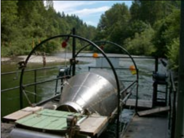
FIGURE 8. — Back end of the screw trap showing the auger cone, live well (covered), and trash drum (Green River, Washington).
