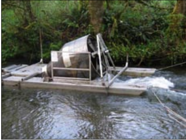
FIGURE 12. — Rotary screw trap outfitted with a single forward winch in the nonfishing position.
