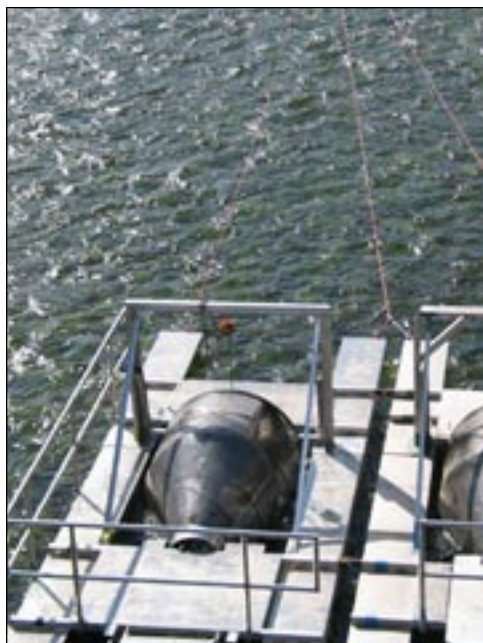
FIGURE 11. — Example of a highline anchoring system for two screw traps operating side by side (Wenatchee River, Washington).
