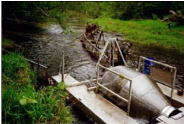
FIGURE 10. — Tripods and screen panels bolted to bedrock substrate to improve screw trap operation in a low-gradient coastal stream.
