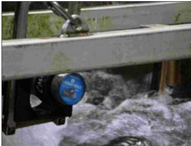
FIGURE 14. — Hub-odometer attached to shaft of rotary screw trap. Hub-odometer readings are used to determine the number of hours the trap fished if trap is stopped by debris when staff is not present.
