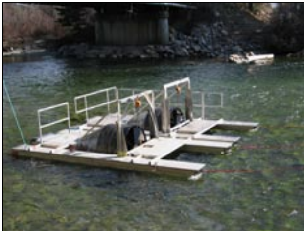
FIGURE 7. — Two rotary screw traps in the nonfishing position suspended from a three pontoon barge (Wenatchee River, Washington).
