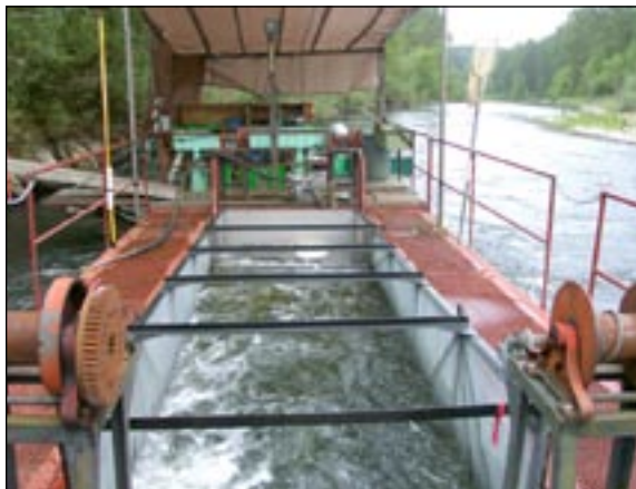
FIGURE 4. — Fishing scoop trap showing the fore and aft winches used to raise and lower the trap, the trap apex, live well, and catch processing station (Chehalis River, Washington).
