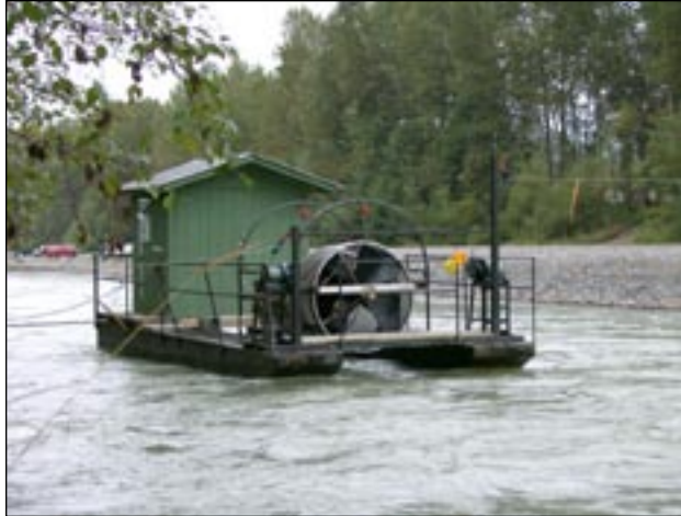
FIGURE 6. — Screw trap mounted on a pontoon barge in the nonfishing position (Puyallup River, Washington).
