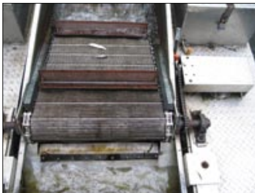
FIGURE 5. — Close-up of a motorized incline plane trap's moving screen with attached cups that help keep juvenile fish from escaping off the screen.
