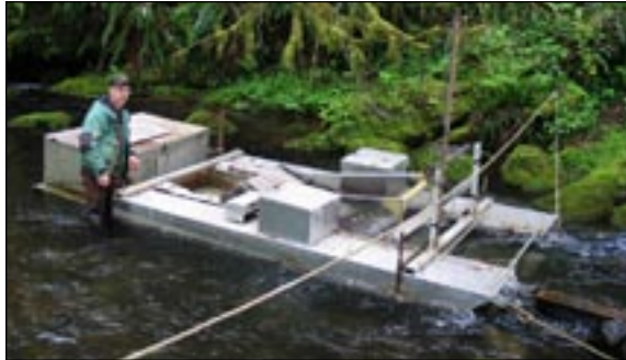
FIGURE 3. — Motorized incline plane trap used in small Oregon coastal streams to monitor downstream migration of juvenile salmonids.
