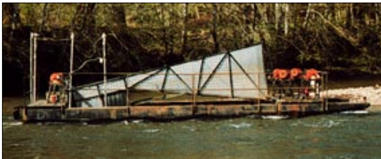
FIGURE 2. — Scoop trap mounted on a pontoon barge, shown in the nonfishing position (Clearwater River, Washington).
