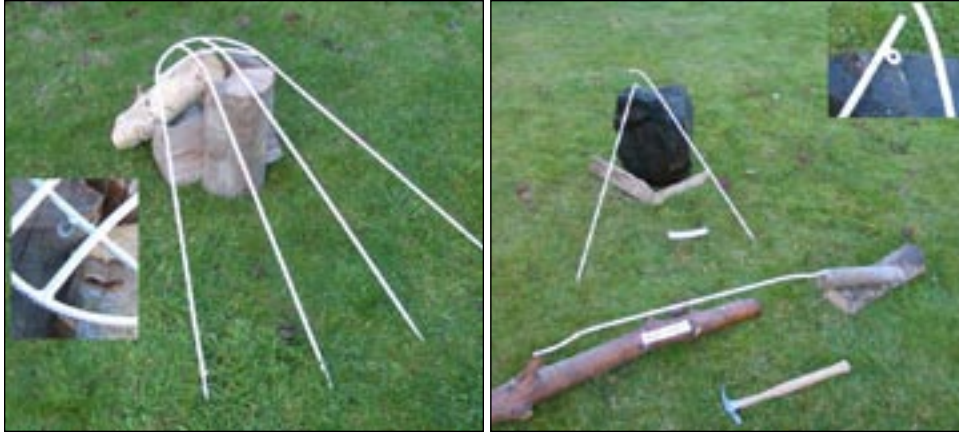
FIGURE 4. — Devices built out of rebar to bridge over rocks, boulders, snags, large woody debris, and so forth, to allow beach seining for capturing adult chinook salmon in the Green River in Washington in 2000–2002: a pitchfork device (left); two J-bar and a bridge (U-bar) devices (right). The insets show placement of welded washers that allow nailing the devices to wood objects. (Photo: Peter Hahn, Washington Department of Fish and Wildlife.)
