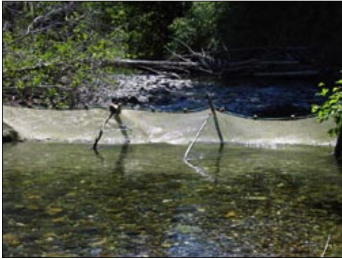
FIGURE 3. — Block nets used to isolate stream section.
